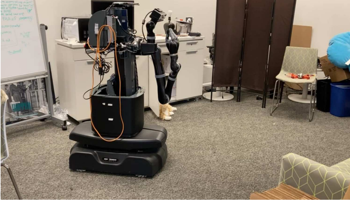
Figure 5.11: Test environment for object search with MOVO using GenMOS. The target object is, again, the toy cat. In this case, it is lying on the floor next to the opened door.
