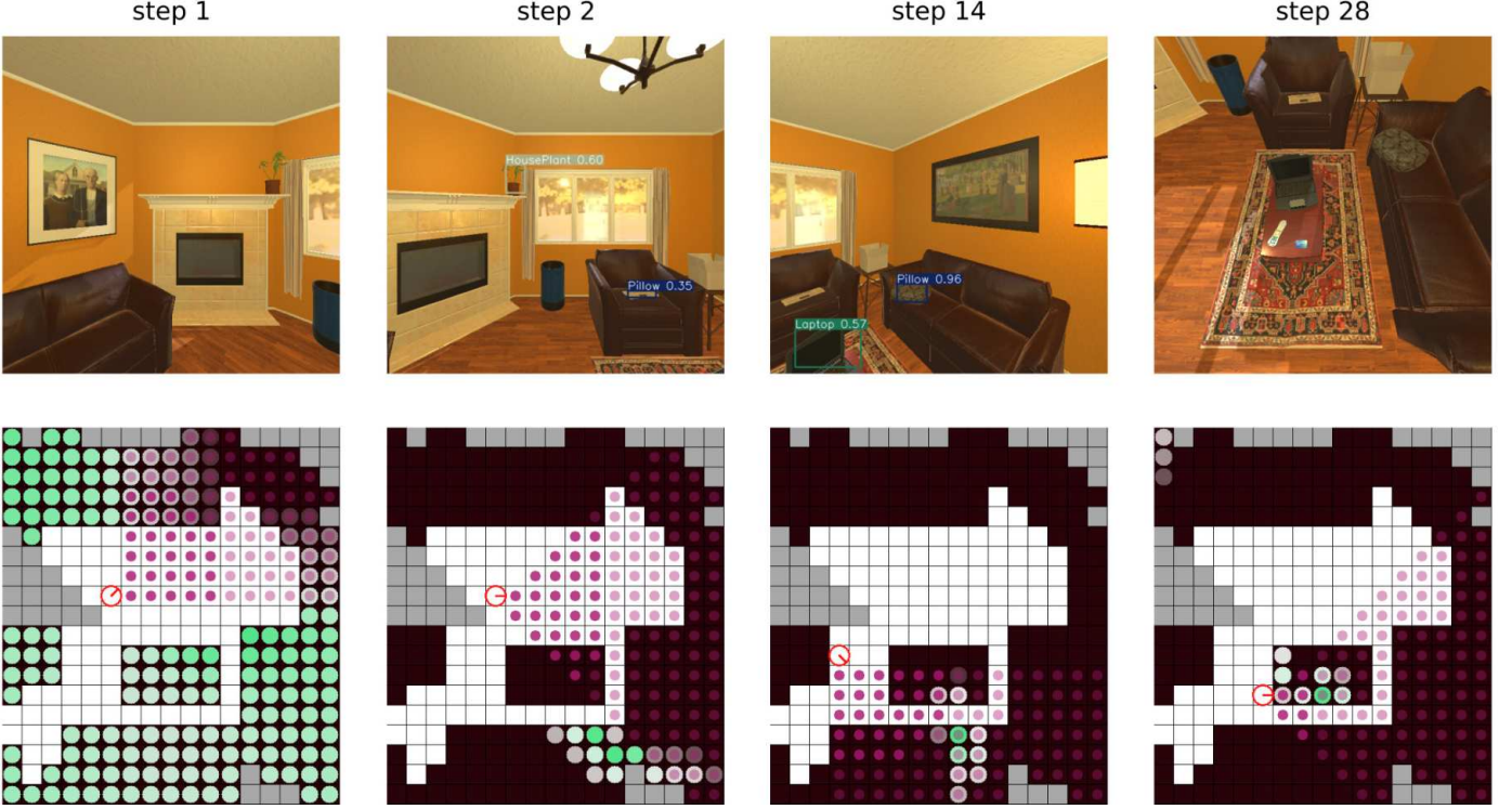
Figure 6.3: Example Sequence. Top: first-person view with object detection bounding boxes. Bottom: Visualization of belief state corresponding to each view. See Fig 7.2 for the legend of the belief state visualization. Our method (COS-POMDP) successfully finds a CreditCard in a living room scene, leveraging the detection of other objects such as FloorLamp and Laptop. For more examples, please refer to the video at https://youtu.be/wd1tmD0mckY .
